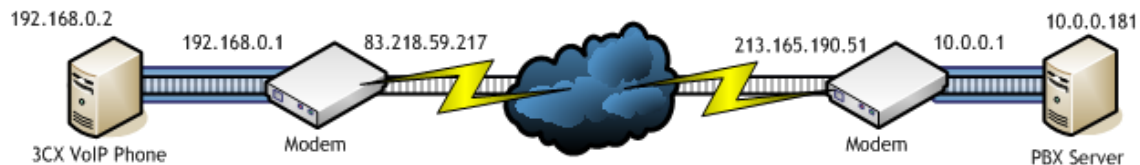
Figure 4 - How a tunnel works
